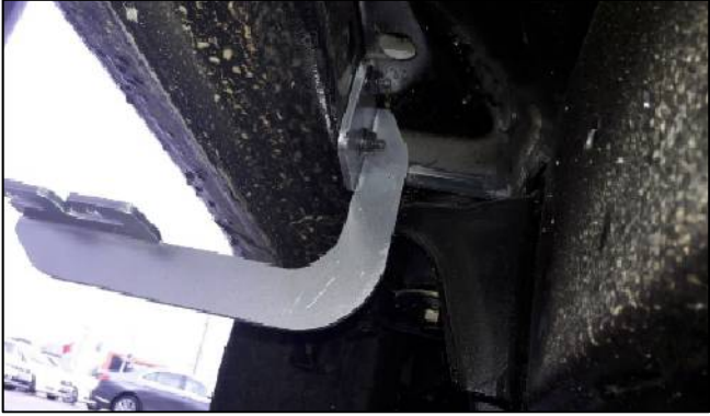
BRAKETİ RESİMDEKİ GİBİ TAKINIZ INSTALL THE BRACKET WITH BOLTS
